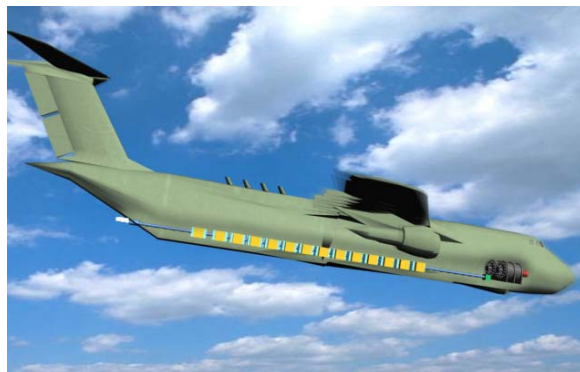
Fig. 1. Airborne launch platform showing a distributed EM launcher for launch to space.
