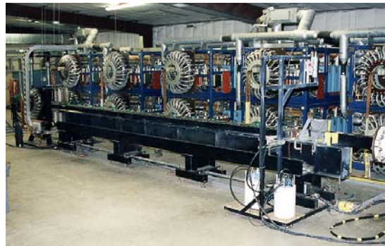
Fig. 3. The existing IAT power supply has 13 independent 1 MJ capacitor modules.
